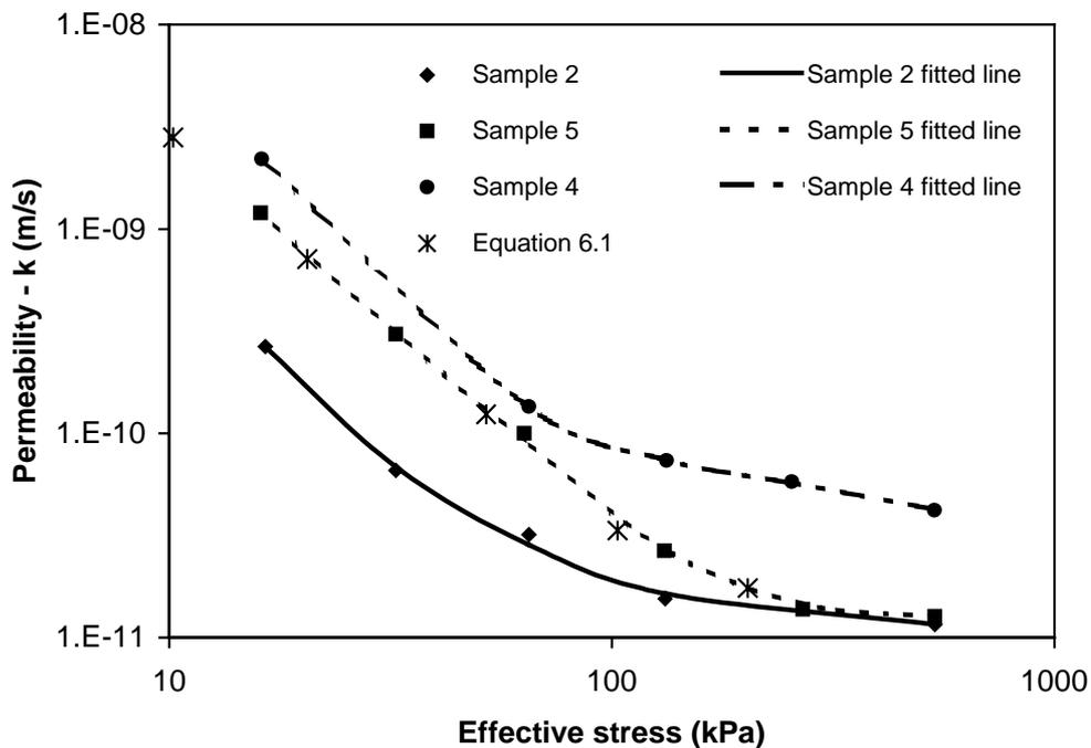
**Figure 6.3.4** Permeability (m/s) as a function of effective stress (kPa) for tailings from the Ranger Mine located 22 km from Jabiluka
