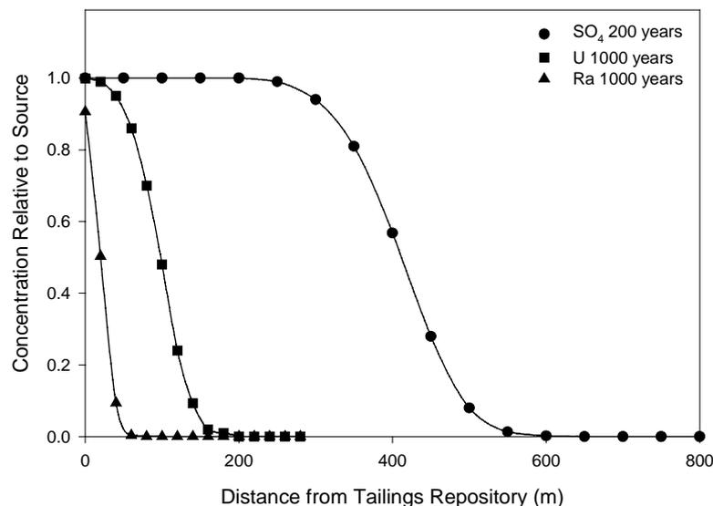
**Figure 6.3.6** Variation of the median concentrations of SO<sub>4</sub>, U and Ra with distance west of the tailings in the mine void at Jabiluka. Concentrations are expressed as ratios to the 'source' concentration immediately downstream of the void. The SO<sub>4</sub> concentrations were calculated 200 years after placement. The U and Ra concentrations were calculated 1000 years after placement.
