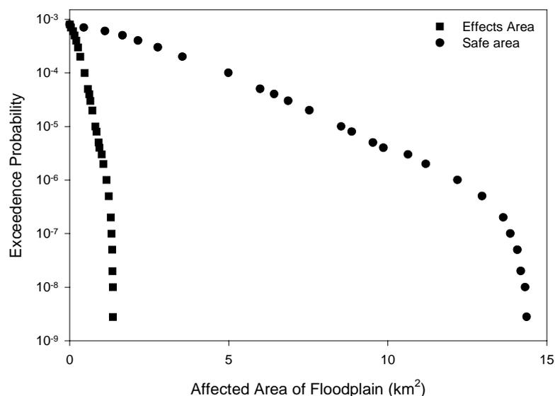
**Figure 5.3.6** Probability versus the affected area of the Magela floodplain for a severe earthquake. Beyond the safe area, no adverse effects are expected. Adverse effects on invertebrates are expected inside the effects area. Between the two areas, some residual effects may occur.
