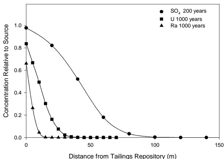
**Figure 6.3.5** Variation of the median concentrations of SO<sub>4</sub>, U and Ra with distance east of the tailings silos at Jabiluka. Concentrations are expressed as ratios to the 'source' concentration immediately downstream of the silos. The SO<sub>4</sub> concentrations were calculated 200 years after placement. The U and Ra concentrations were calculated 1000 years after placement.
