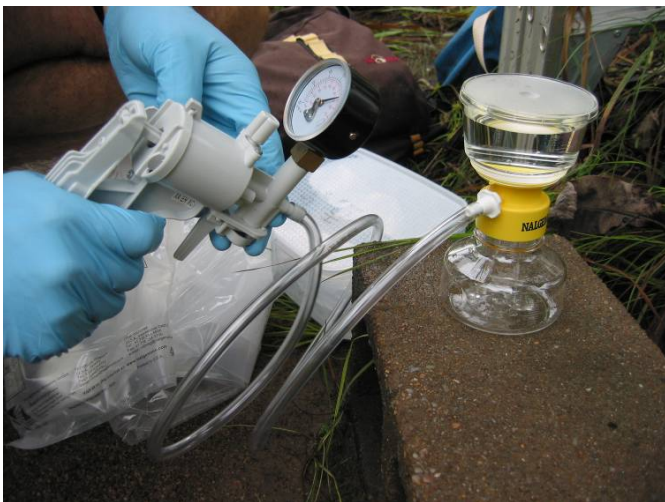
Filtering a water sample in the field immediately after collection helps to preserve the sample for chemical analysis.
