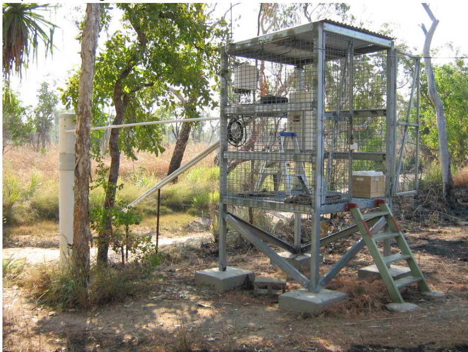
A continuous monitoring station measuring electrical conductivity, turbidity, pH and water level on the bank of Gulungul Creek. The station is also equipped with an automatic water sampler.
