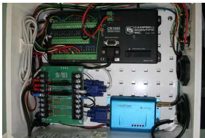
The logger system controlling the measurement sensors and recording the data at a continuous monitoring station. The information is transmitted via mobile phone link to Darwin
