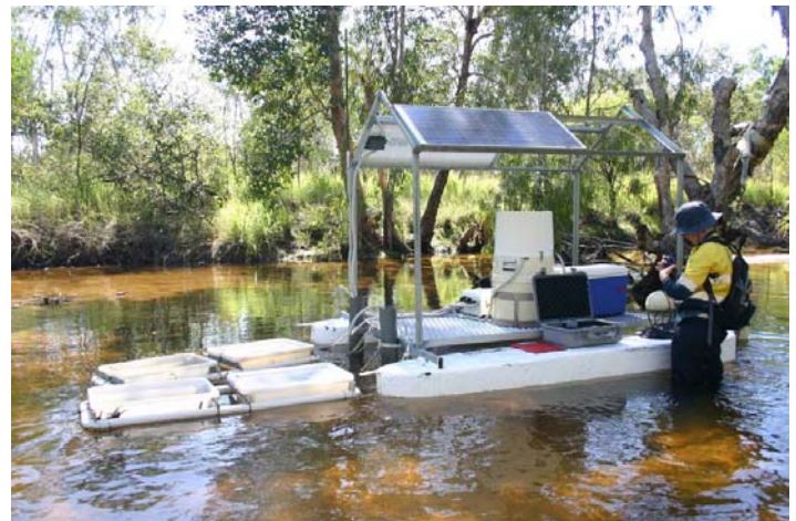
A continuous monitoring station measuring EC, turbidity and pH on a pontoon in Magela Creek. The pontoon also has an automatic water sampler and tubs (floating in water at rear) containing snails for in-situ snail toxicity testing.
