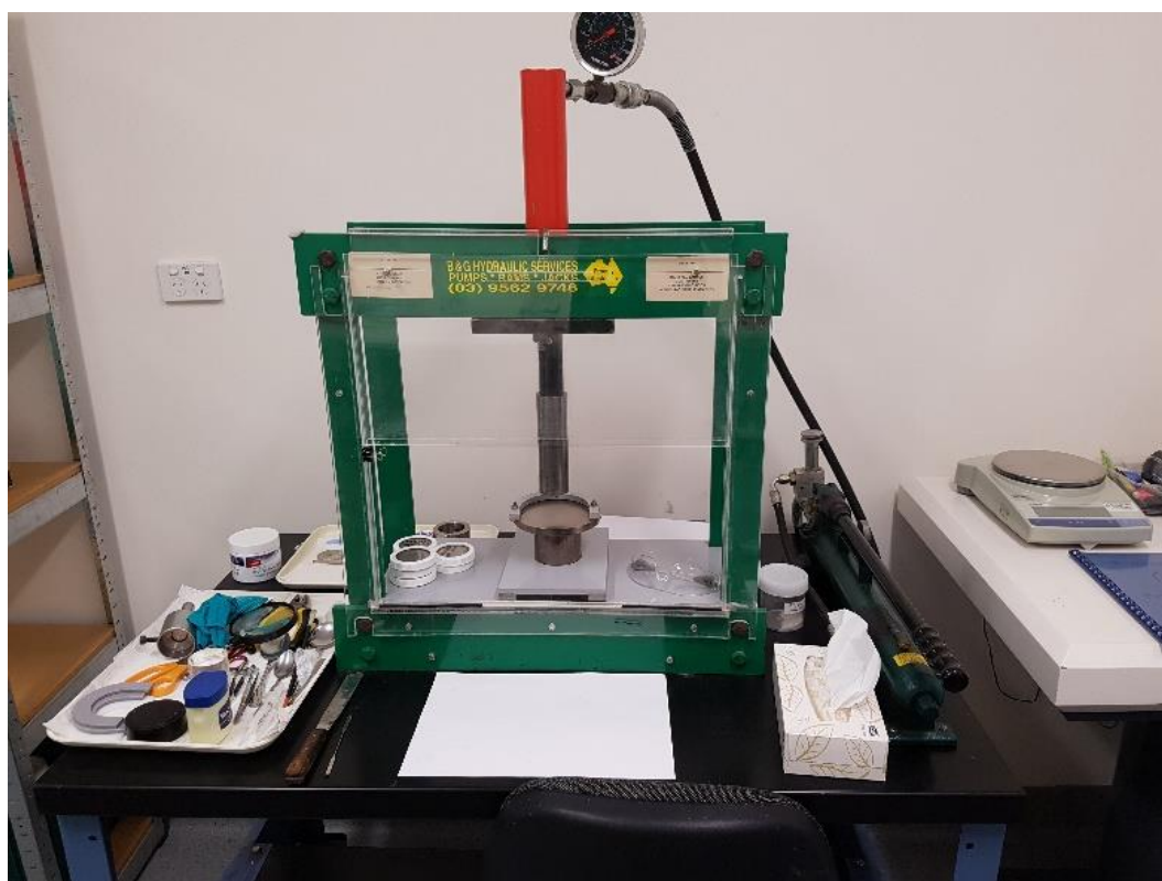
Figure 3 Hydraulic press for compressing sample material into acrylic containers.
