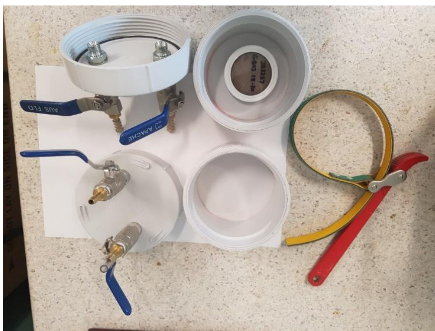
Figure 6 Test chamber base, lid with o-ring and inlet and outlet ports, with flexible oil filter wrench to assist in sealing the chamber.
